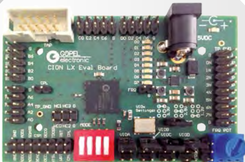
CION-LX Evaluation Board enables evaluation of all CION-LX operation modes and features
