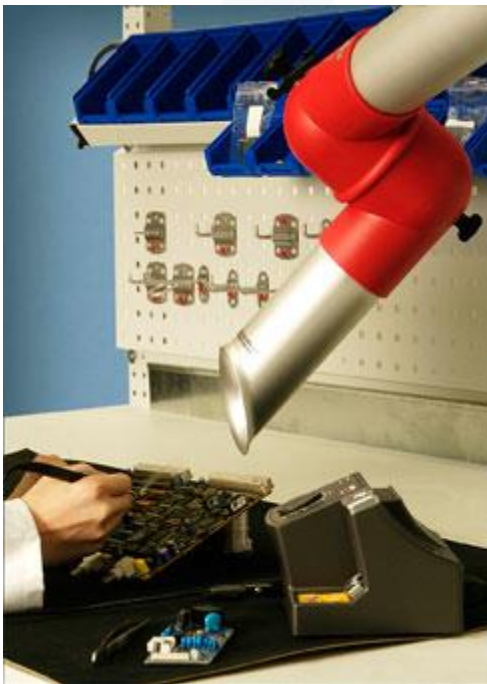
Image 4: Soldering fume extraction at manual workplace – Utilisation of a suction pipe mounted on an extraction arm
